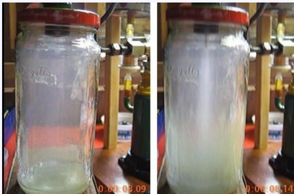
If you have Bosch DN 0 SD 240 nozzles with the hole-type pintle, an initial jet sprays out the hole in the pintle prior to the actual spray – if you have these nozzles and see this jet, it isn't a sign of a malfunctioning injector! This can sometimes be hard to test for; I found it worked well to build the pressure really slowly and carefully – this lets you see the initial jet before the pressure gets high enough that the injector pops.
